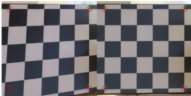
Figure 4: The affine transformation of the images of Fig.3. Points A, B, and C on the checkerboard got mapped to the corresponding arbitrary points marked with red circles. Image by the author.
